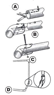
Insert the push-button springs into drilled PVC sections (side bars) as shown in Diagram A.
